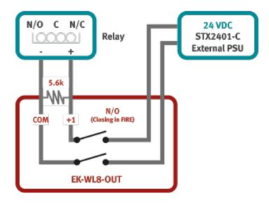
The external PSU will supply the voltage to the power terminals of the Ekho Output Module (rated for 250 VAC but we would recommend only using VDC). When the fire alarm is activated, the Output Module will switch the voltage by closing the two contacts.
