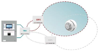
If the signal to Expander 1 is compromised, the sensor automatically finds and connects to an Expander with the next strongest signal pathway, in this example, Expander 2.
