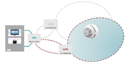
In this example, the Ekho sensor is connected to the Translator via Expander 1, as it is the strongest signal pathway.
