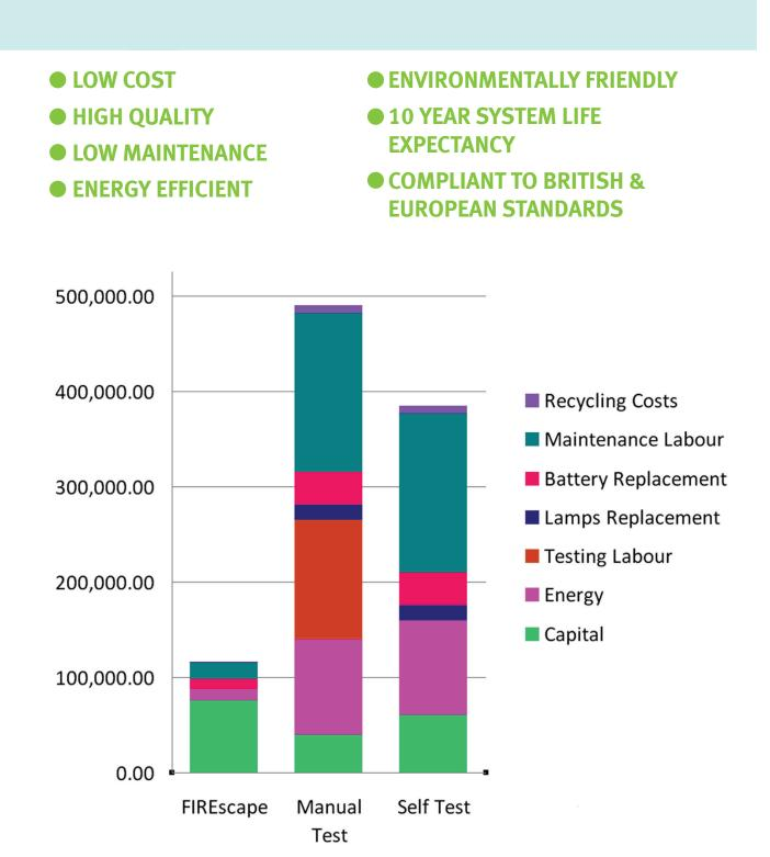
Total cost of ownership comparison based on a 1000 luminaires, 80% non-maintained, 20% maintained, emergency lighting system for manual-test, self-test and Hochiki's FIREscape system, over a 10 year period.
