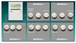
Short circuit isolators (either on the loop or within the CIE) should be installed to limit the loss of fire cover caused by a single fault to **2000m**<sup>2</sup>. The loss of fire cover caused by two simultaneous faults should be limited to **10,000m**<sup>2</sup>. This will therefore restrict the cover provided by any analogue loop to **10,000m**<sup>2</sup> maximum.
