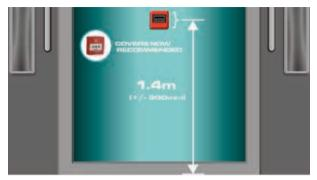
Manual Call Points should be positioned **1.4** (+/-**300** mm) from finished floor level and if sited below **1.1** m a variation will be required. They may be They may be semi-recessed if readily visible but if required to be seen from the side (for example, in a corridor) they should be **15** mm proud of the wall.
