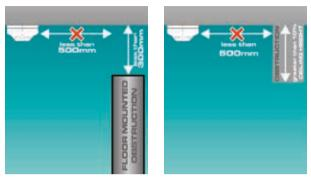
Ceiling obstructions, if deeper than **10%** of the ceiling height, or floor mounted obstructions (e.g. partitions) where the top is less than **300mm** from ceiling should be treated as walls. No detection device should be mounted within **500mm** of any wall or obstruction treated as a wall.
