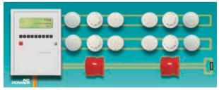
Cables used for the Critical Signal Path and the final LV (low voltage) mains supply to any fire detection equipment are now required to be fire resistant and coloured externally in a single, common colour (red is preferred). The LV supply to all parts of the system should be provided with a double pole, lockable isolation device for the safety of the maintainer. Non-critical cabling may still be non-fire resistant, for example door retainer circuitry which may fail to safe.
