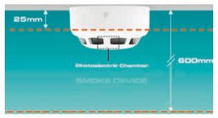
The sensing element of a Smoke detection device (photoelectric chamber) should not be less than **25mm** below the ceiling, and not greater than **600mm** below the ceiling.
